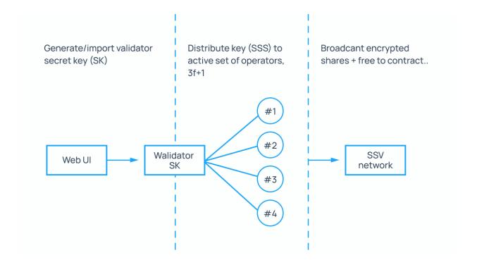
Instead of running a single validator instance susceptible to technical issues, hacking, and high maintenance costs, with SSV a DIY staker can run their validator in a decentralized manner while still having full control over their validator keys.
